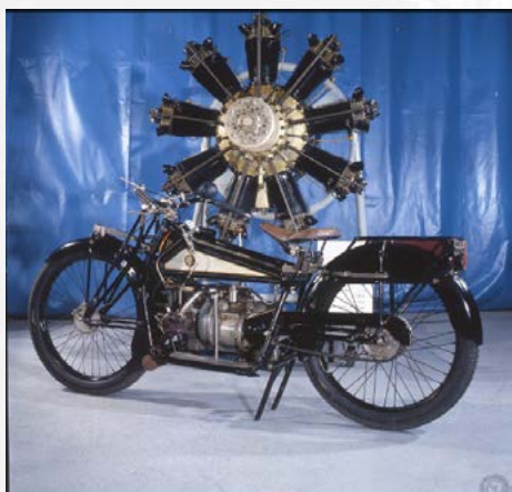
1922 Gnome & Rhône ABC/Type A. Nine-cylinder 60 HP rotary engine – the last operational radial engine of this type built in 1920 Photo credits: moto-collection.org François Marie Dumas
